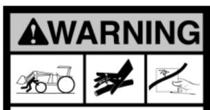
Raised loader or boom can fall from hydraulic system failure. To avoid serious injury or death:
